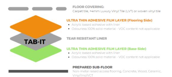
The following is a guide on how to install carpet tiles, +4mm Luxury Vinyl Tiles (LVT) and woven vinyl tiles onto receptive bases in various configurations using IOBAC Tab-It.
