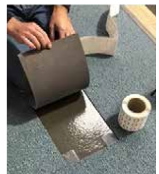
Comparison of uplifting a tile installed with adhesive (above) vs IOBAC
